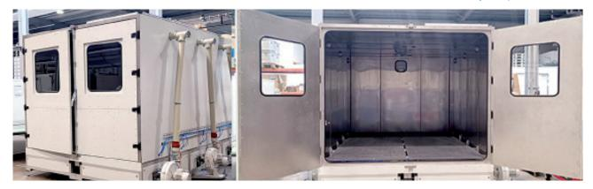
Testing the reliable function and safe use of a device or component includes leak testing and testing for ingress of foreign bodies and dust. The exposure of various devices to dust can also be simulated. In many standards, dust tests are mandatory and are a component of several tests that a DUT must pass before being launched to the market.
