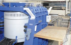
VIBRATION – with climatical and electrical overlay – 300 kN Shaker
